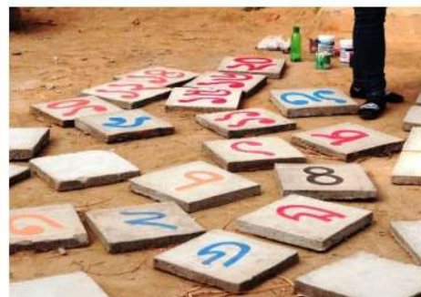
Everything was made locally, the square paves were made combining local knowledge and advanced knowledge of the use of a wired mesh to make it stronger for heavy use by children
